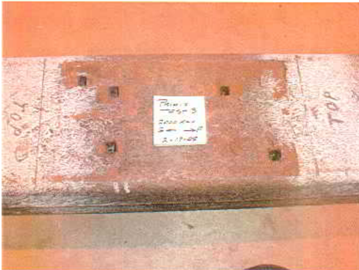
Figure 4. Shows no significant tie plate cutting or plate area deformation after 2-million cycles
