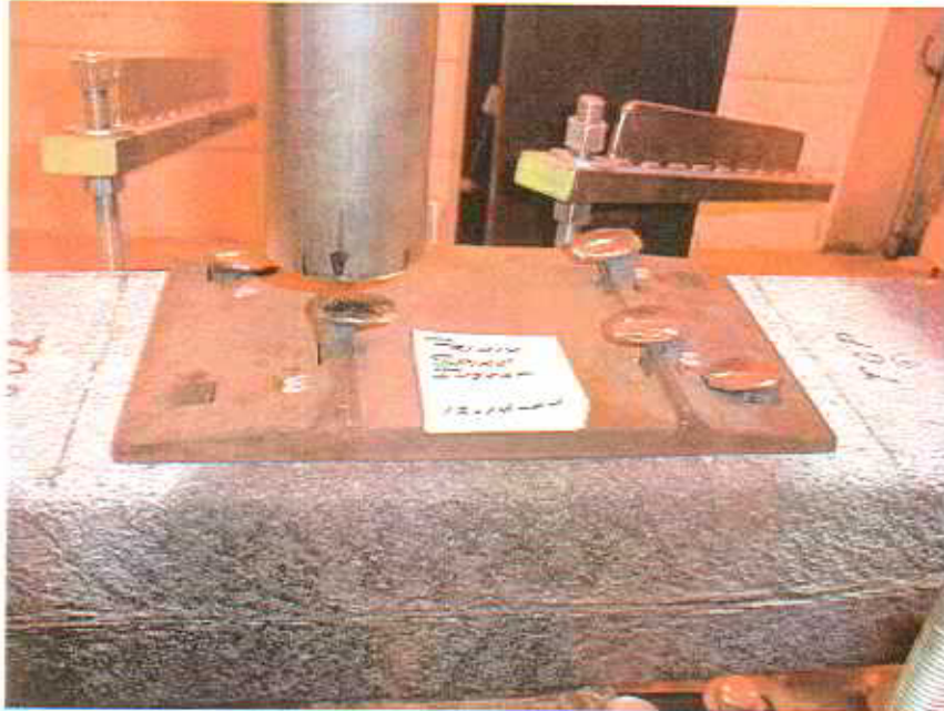
Figure 1. Cut spikes were inserted without pilot holes using a hydraulic press
