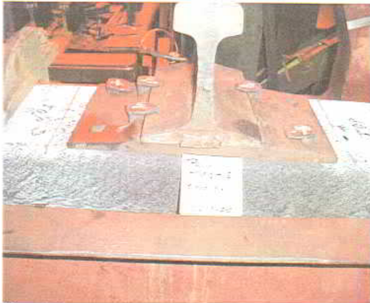
Figure 3. Post test photograph shows no significant cut spike uplift after 2-million cycles
