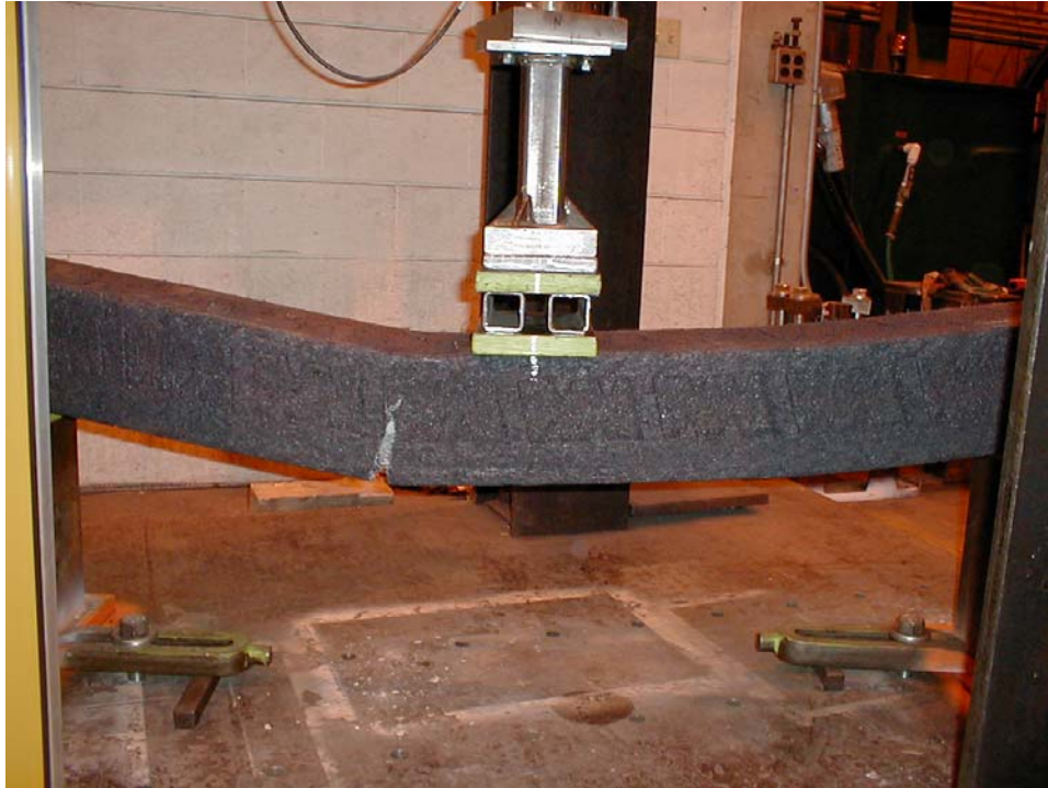
Figure 7. Tie Loaded to Failure
