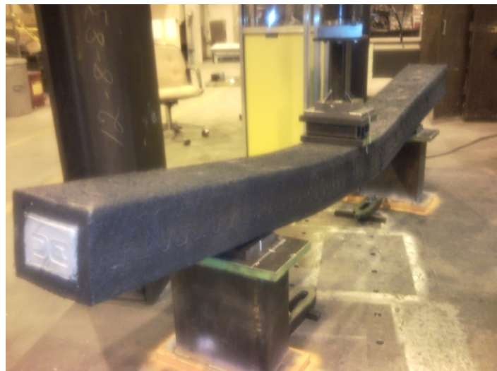
Figure 5. Tie Loaded to Failure
